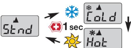
The display then changes over to the "Weather correction mode". When the Victorinox emblem is pressed briefly, the correction setting can be altered in the sequence "Std", "Cold", "Hot".
