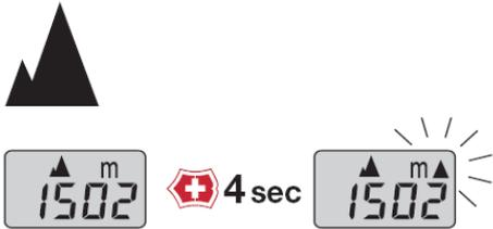
Press the Victorinox emblem for **4** seconds until the display flashes. Now release the Victorinox emblem again. You have changed over to the altimeter setting mode.
