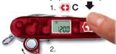
To set the American system of units (height = ft, temperature = °F, time mode = 12h), press the Victorinox emblem while closing the battery compartment. The function test then takes place as described above.
